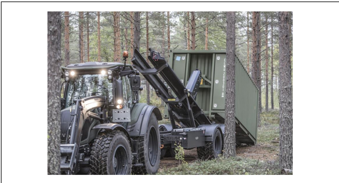
Figure 2.1 4WD heavy-duty tractor with hook-trailer bearing containerised unit in the general configuration proposed for PFP 2 mobile training units.
