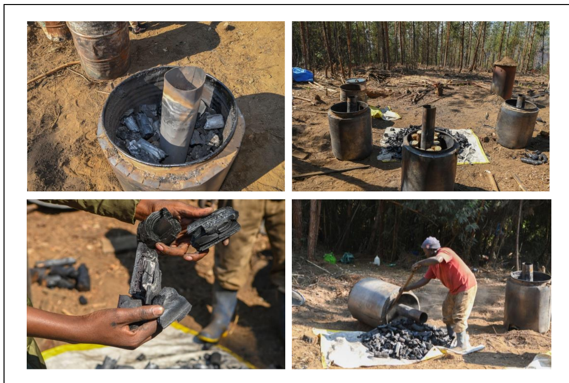
Figure 2.8: A modified oil drum kiln for small scale charcoal production
