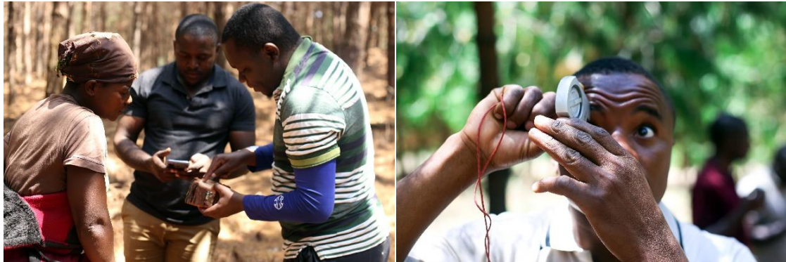
Figure 3.7 Fieldwork for woodlot assessment: Calculation of annual rings for stand age (left) and measurement of tree height (right)
