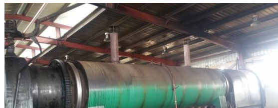
Fig 8 Mkaa Endelevu pyrolyzer (most advanced technology in Tz). Recovery rate: 30-40%. Production capacity: 20 tons of biochar per day
