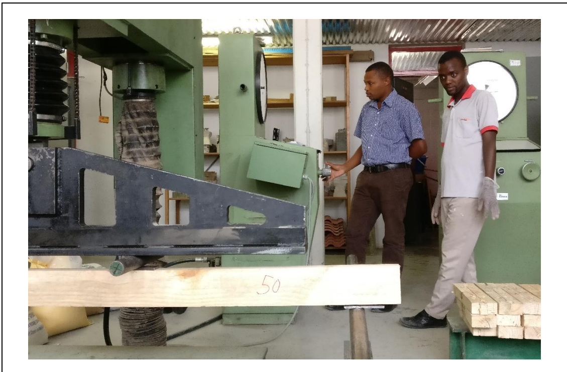
Figure 6 Destructive testing (shear) done at TBS for establishing the strength values of sawn wood
