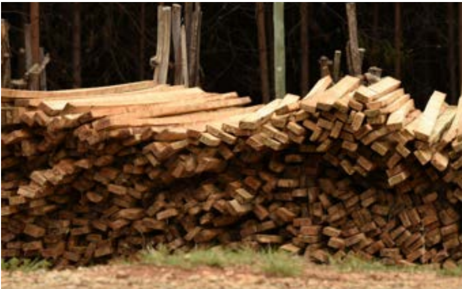
Improper technique of timber seasoning
